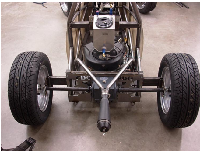
Rear axle, with the exhaust, gear box, muffler, and back plate.
